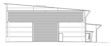
T-model, where the middle part can be used as a passage opening, and when fully raised, the crane can be driven out.
